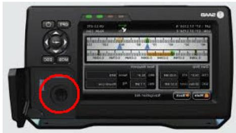
or via wired Pilot Plug AMP "Male" connector at the Pilot operation place:
